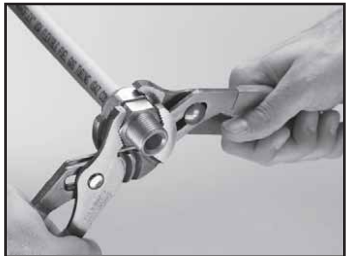
Step 4 Tighten with wrenches until nut contacts body.
