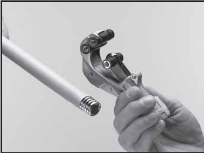
Step 1 Cut WARDFLEX tubing and remove Polyethylene coating to expose a minimum of four corrugations.
