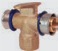
Viega PEX Press tee Zero Lead - For fire sprinkler systems - Bronze - Press connection, female pipe thread - Mounts to horizontal surfaces Note For use with black ViegaPEX Ultra only. UL listed for NFPA 13D systems Model 2818.2ZL
