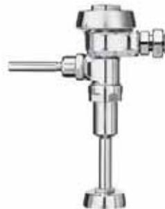
Urinal Flushometer with Adjustable Ground Joint Tailpiece for ¾" Top Spud MODEL 188 XD (0.13 gpf/0.5 Lpf) MODEL 188 XD (0.25 gpf/1.0 Lpf)
