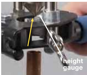
3. Insert tubing until it touches the height gauge
