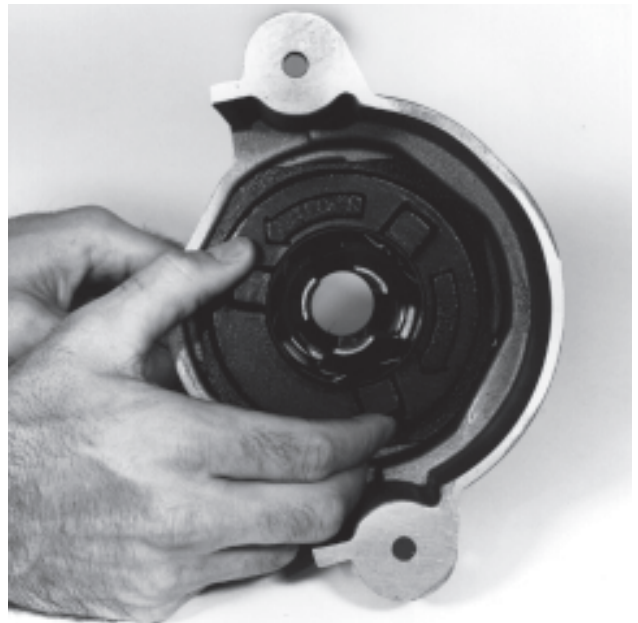
Figure 12 – Remove Jaw Set Cover
