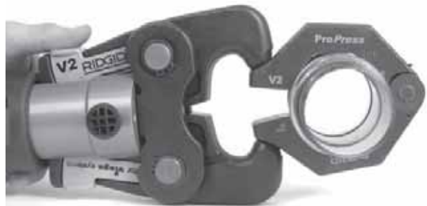
Figure 9 – Attaching Actuator to Press Ring
