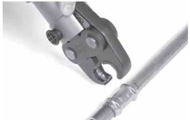
Figure 6 – Opening The Scissor-Style Jaw Set
