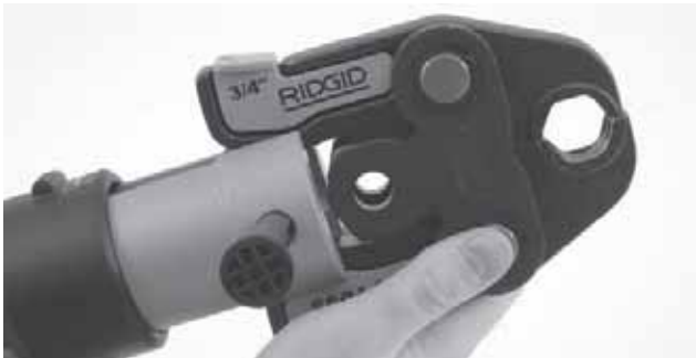
Figure 5 – Slide Attachment Into Tool
