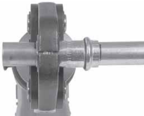
Figure 7 – RP 340 Tool Square To Tubing
