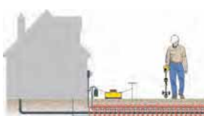
Direct connect to utility lines.
