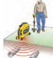
Induce a signal to locate utilities.
