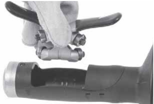
Figure 12B – Removing AUTOFEED Mechanism From Housing
