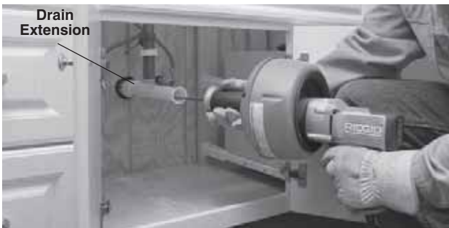
Figure 6 – Example Of Extending Drain To Within 6" (15cm) Of Drum Opening
