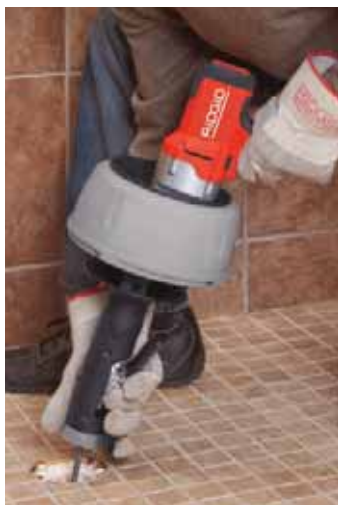
The \frac{3}{8} " cable in Model K-45AF-5 and K-45AF-7 extends machine's capacity to 2 \frac{1}{2} " drain lines.
