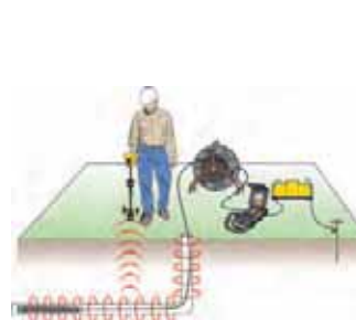
Find plastic pipe with integral line trace.
