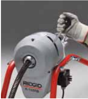
Engage clutch, cable spins
