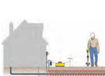
Direct connect to utility lines.
