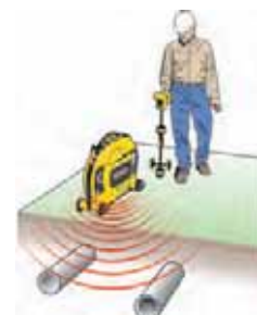
Induce a signal to locate utilities.
