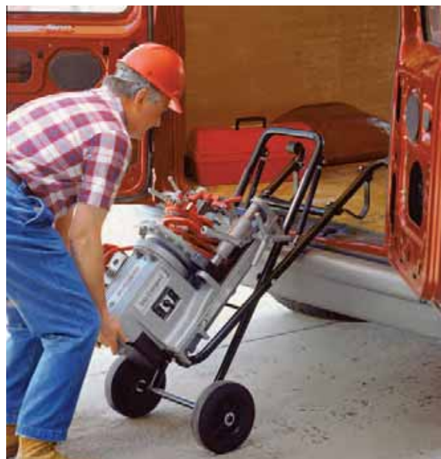
Model 300 Compact is a versatile choice for threading and roll grooving applications.
