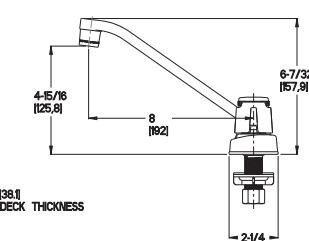
Ø1-3/8 Min to Ø1-1/2 Max. Deck Hole Openings
