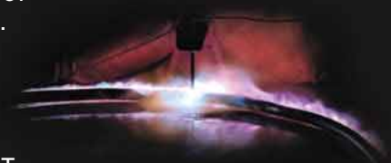
Simulated lightning test with no product failure
