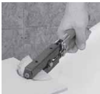
Notcher may then be used to cut all the way through plank along pre-scored line.
