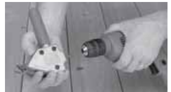
The camshaft of the TURBOSHEAR inserts directly into the 3/8" chuck of a standard 1200 rpm A/C or cordless drill.
