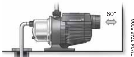
Fig. 3 Minimum clearance behind the pump
