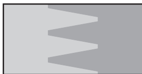
Regular pipe threads, hand tight. Only seals joints on the sides of the threads, allowing spiral leakage.
