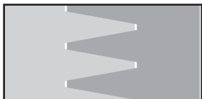
Regular pipe threads, hand tight. Only seals joints on the sides of the threads, allowing spiral leakage.
