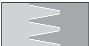
Dryseal pipe threads, wrench tight. Tightly seals all thread surfaces, providing a positive seal.
