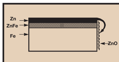
Protection of cut edges with zinc coatings.
